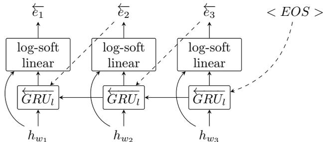
FIGURE 2 – Structure of the backward decoder
